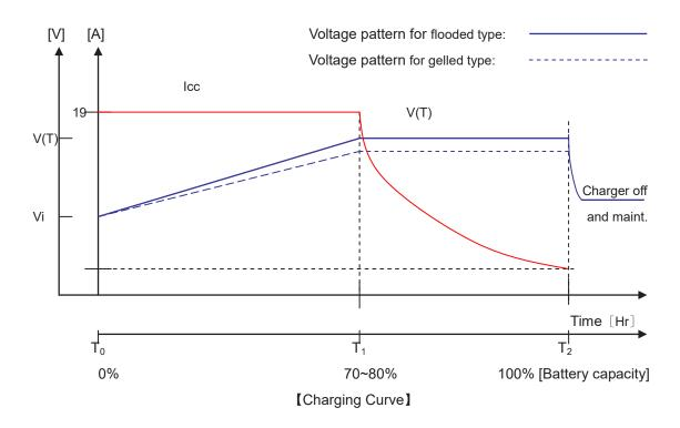
Voltage Vi is initial battery voltage when battery is connected with charger.
