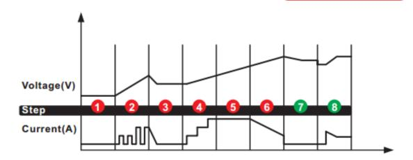
STEP 1: DIAGNOSIS (Check if battery has connected with the charger and also check battery voltage)
